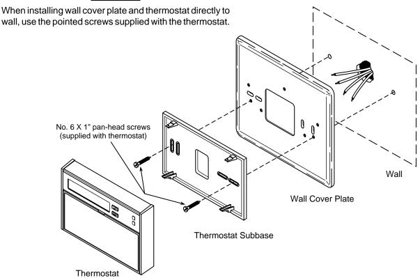
Figure 3. Mounting 1F9X digital thermostat to wall
